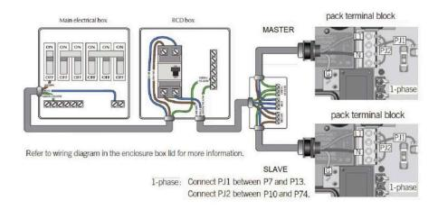
230 VOLT 50 Hz THREE PHASE RCD WIRING (DUAL SPA PACKS)
