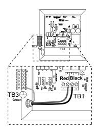
Figure E 120V/240V 60 Hz Convertible Models
